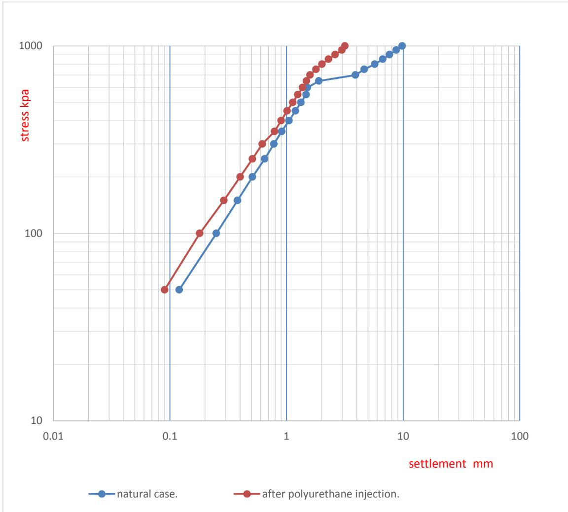
Figure 11. Stress - settlement curve for Mallawi western desert road site with PU injection ratio 10.4 %.
