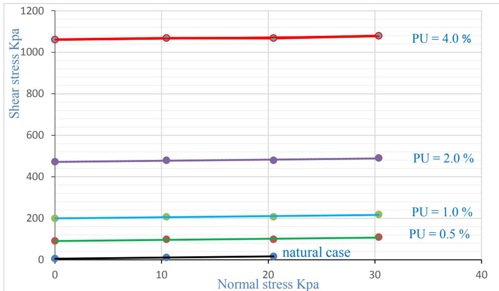
Figure 19. Shear strength parameters of Village 8 - El Minia conditioned samples with different PU% mix ratios.
