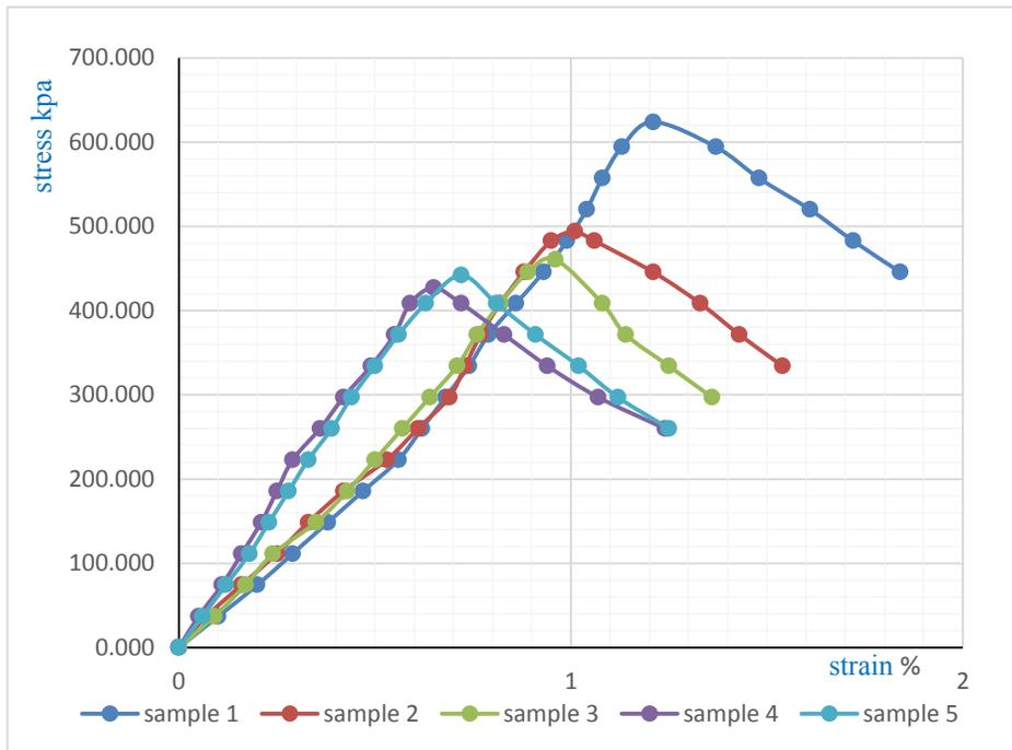
Figure 16. The unconfined compressive strength- strain results of Village 8 -El Minia samples with a P.U. mix ratio of 1.0 %.
