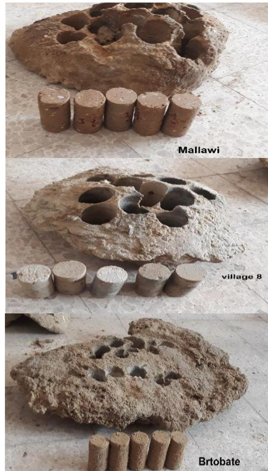
Figure 6. Cylindrical samples extracted from polyurethane conditioned masses.
