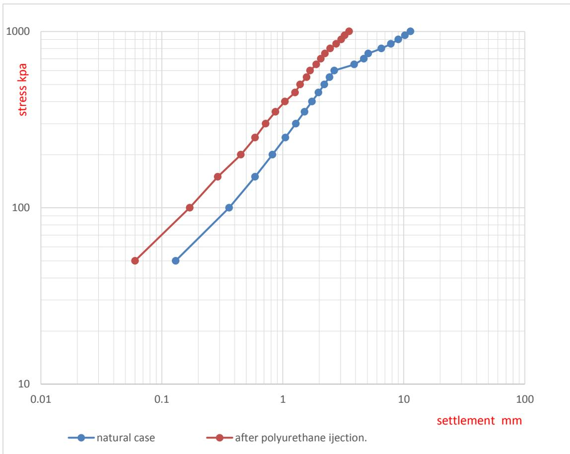
Figure 10. Stress - settlement curve for Village 8 - El Minia. site with PU injection ratio 9.3 %.
