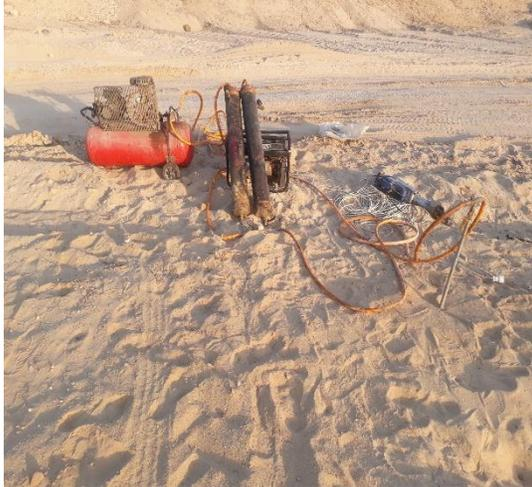
Figure 2. Polyurethane injection set up.
