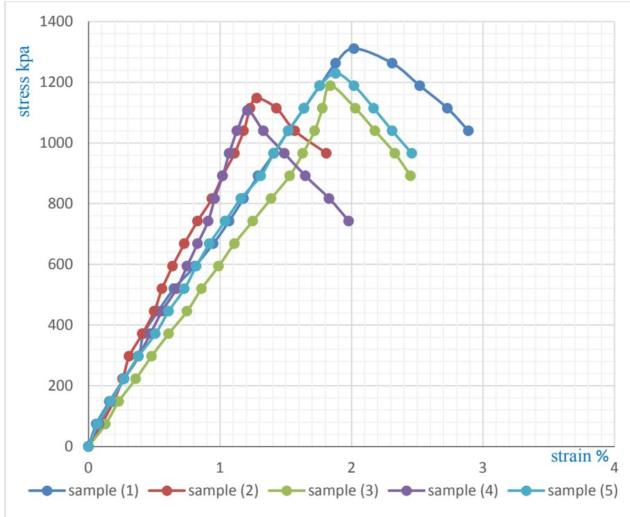
Figure 17. The unconfined compressive strength- strain results of Village 8 -El Minia samples with a P.U. mix ratio of 2.0 %.
