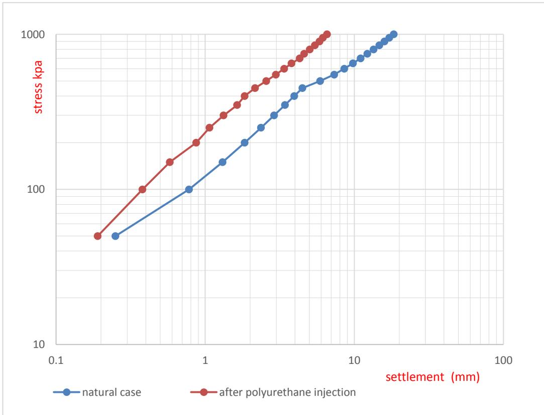
Figure 9. Stress - settlement curve for Brtobate- Maghagha site with PU injection ratio 7.9 %.
