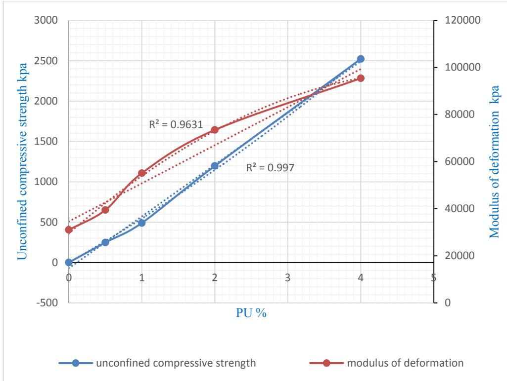
Figure 20. Unconfined compressive strength and modulus of deformation for Village 8 - El Minia conditioned samples with different PU % mix ratios.
