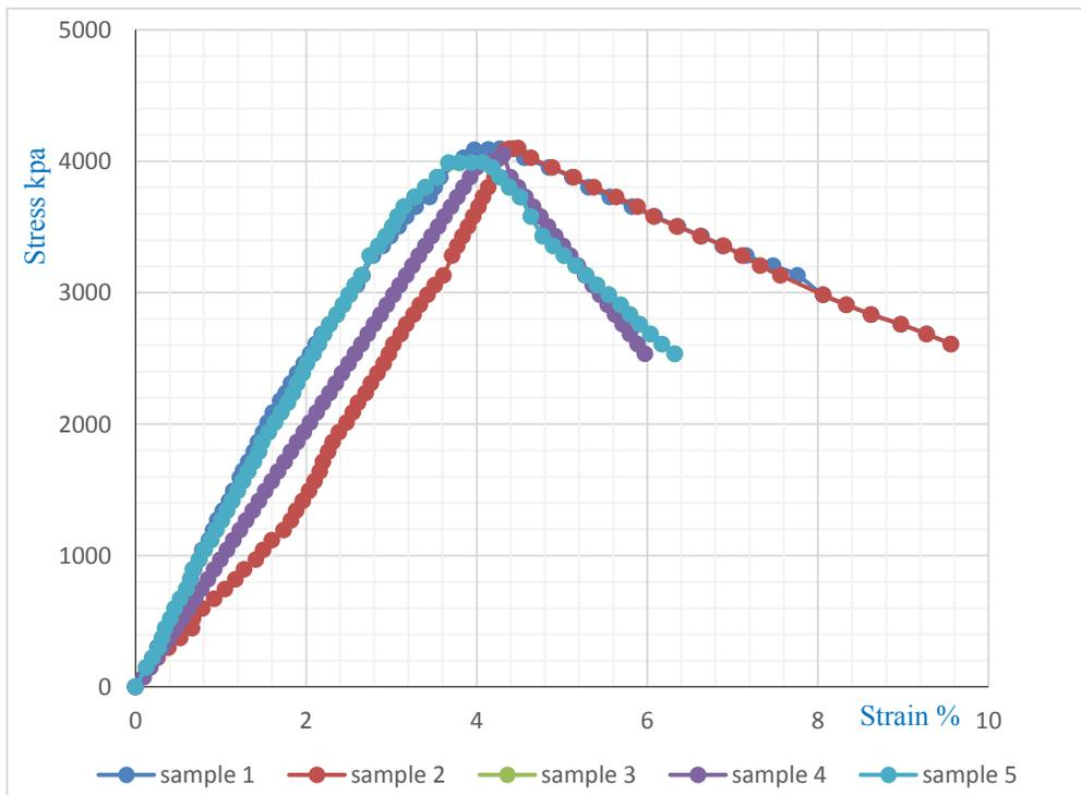
Figure 14. Stress strain curve of Mallawi - western desert road samples with PU injection ratio 10.4%.
