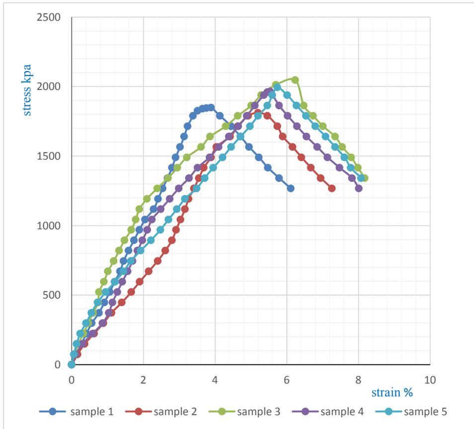
Figure 12. Stress- strain curve of Brtobate - Maghagha samples with PU injection ratio 7.9%.
