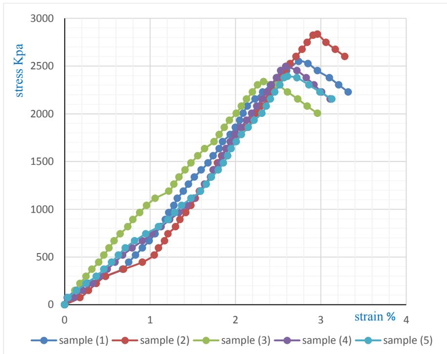
Figure 18. The unconfined compressive strength- strain results of Village 8 -El Minia samples with a P.U. mix ratio of 4.0 %
