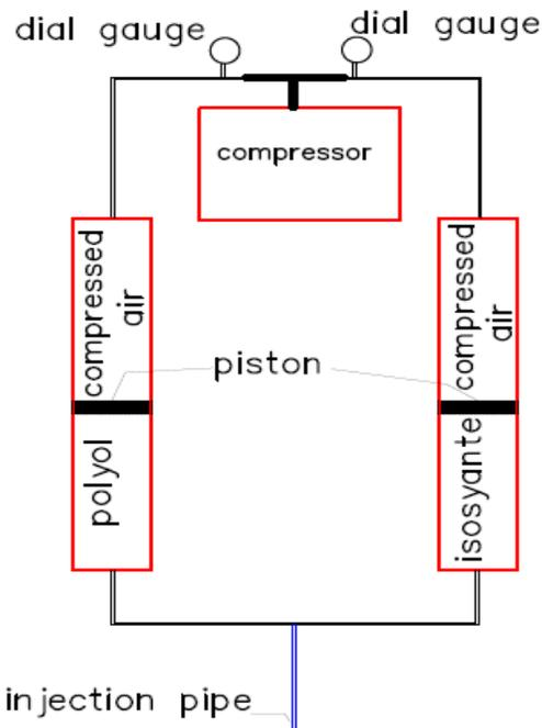
Figure 3. A schematic diagram for the injection set up..
