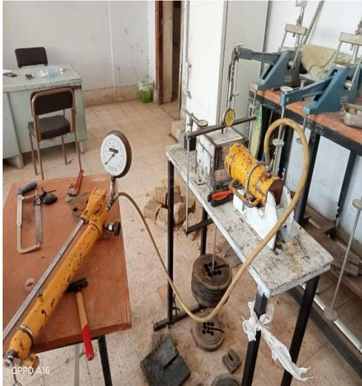
Figure 8. Fabricated direct shear device.
