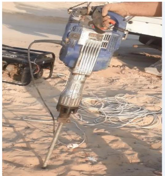
Figure 4. Electric drill to drive injection pipe into sand.
