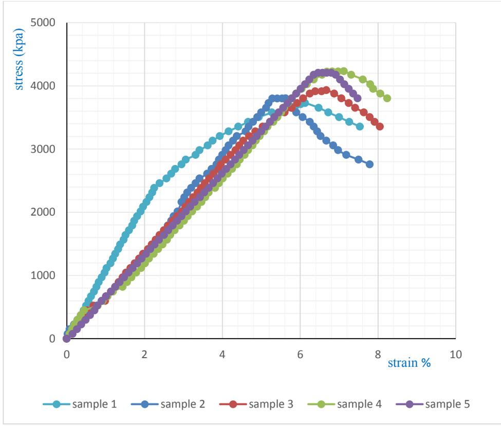
Figure 13. Stress strain curve of Village 8 - El Minia samples with PU injection ratio 9.3%.
