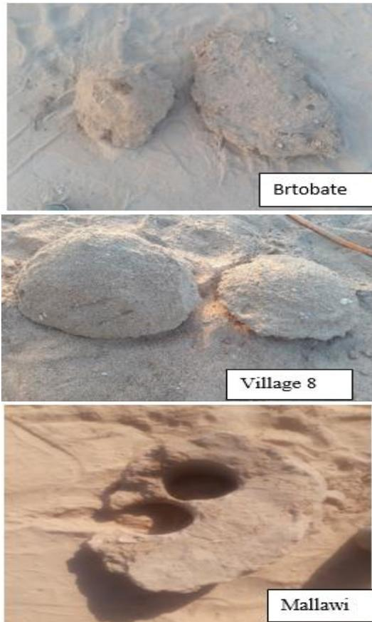
Figure 5. Polyurethane injected sand mass from three sites.
