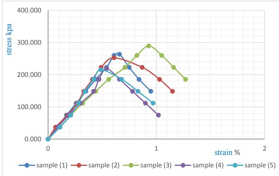
Figure 15. The unconfined compressive strength- strain results of Village 8 -El Minia samples with a P.U. mix ratio of 0.5 %.
