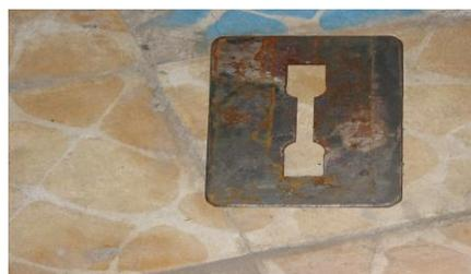
**Figure 2: A Special Stamp for Controlling the Thickness of the Adhesive Material**
