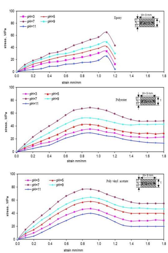
**Figure 9: Effect of pH Values at 4 hrs. on Stress/ Strain Diagram of PVC /PVC Sandwich plates ( $h_2 = 2.5$  mm, 0.95 Wt. % Glass Fiber)**
