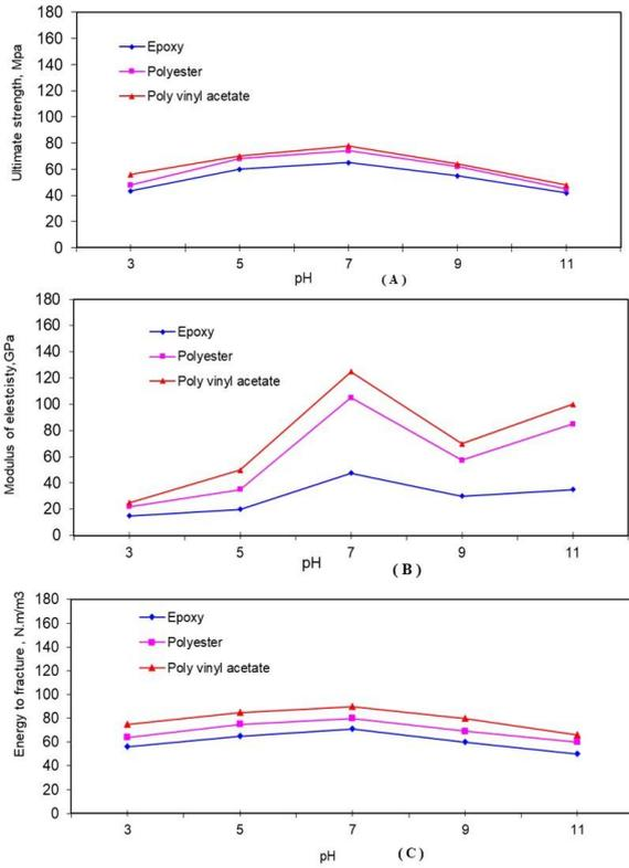
**Figure 11: Ultimate Strength, Modulus of Elasticity and Energy to Fracture Mechanical Tests for the PVC / PVC Sandwich Plates with 0.95 Wt.% Glass Fiber and 2.5 mm from Different Adhesives Thicknesses as a Function of pH Effect at 2 hrs.**
