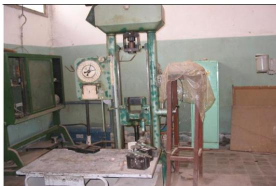
**Figure 5: Adhesion Shear Test Device**
