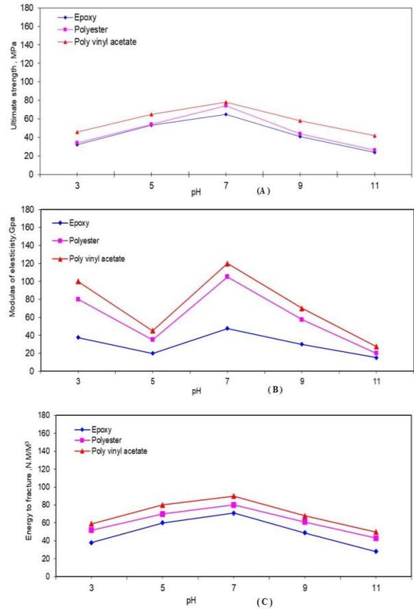
**Figure 12: Ultimate strength, Modulus of Elasticity and Energy to Fracture of PVC / PVC Sandwich Plates with 0.95 Wt.% Glass Fiber and 2.5 mm from Different Adhesives Thicknesses as a Function of pH Values at 4 hrs.**
