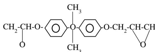
The epoxy adhesive material was brought from the Chemicals for Modern Building Company and it consists of two main components, these components are solvent free and non-pigmented liquid. It is prepared by mixing the hardener with resin at ratio of 1:2, The epoxy adhesive material will dry after 24 hrs. on the PVC sandwich plates
