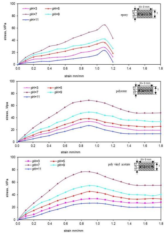
**Figure 10: Effect of pH Values at 6 hrs. on the Stress /Strain Shape of PVC / PVC Sandwich Plate. (  $h_2 = 2.5$  mm , 0.95 Wt. % glass fiber)**
