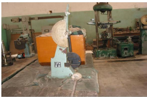
**Figure 6: Impact Test Device**
