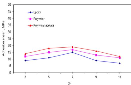
**Figure 17: Effect of pH Values on Adhesion Shear of PVC / PVC Sandwich Plates with 0.95 Wt.% Glass Fiber and 2.5 mm from Different Adhesives Thicknesses at 2 hrs.**
