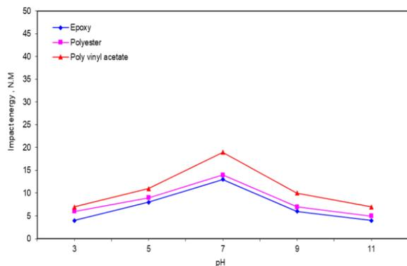
**Figure 16: Effect of pH Values on the Impact Energy of PVC/PVC with 0.95 Wt.% Glass Fiber and 2.5 mm from Different Adhesives Thicknesses at 6 hrs.**
