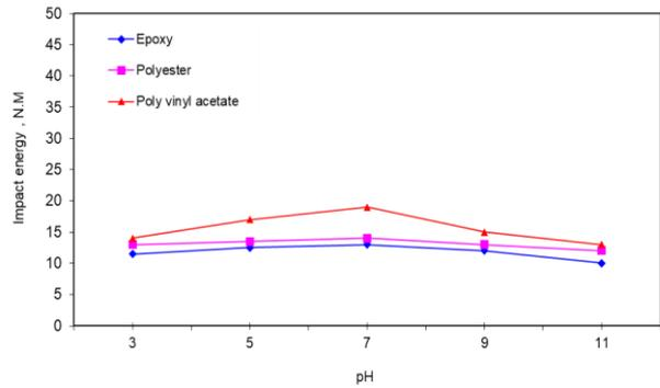
**Figure 14: pH Values Effect on the Impact Energy Test of PVC/PVC Sandwich Plates with 0.95 Wt.% Glass Fiber and 2.5 mm from Different Adhesives Thicknesses at 2 hrs.**
