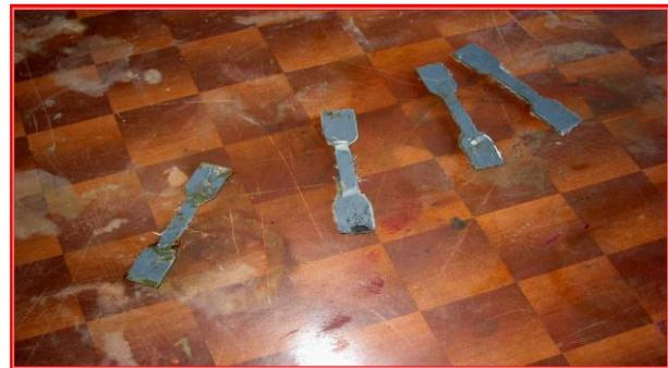
**Figure 3: PVC Specimen for the Tensile Test Applications**
