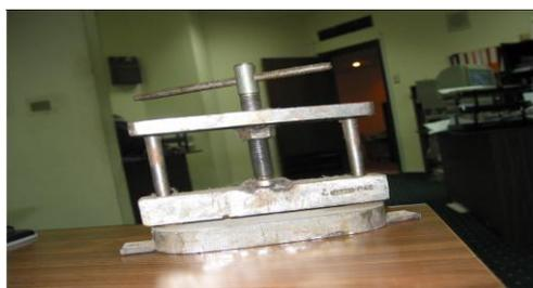
**Figure 1: A special Device for Controlling the Thickness of the Adhesive Material**
