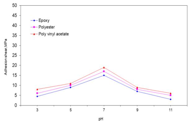
**Figure 19: Effect of pH Values on the Sheer Force of PVC/PVC with 0.95 Wt.% glass fiber and 2.5 mm Different Adhesives Thickness at 6 hrs.**
