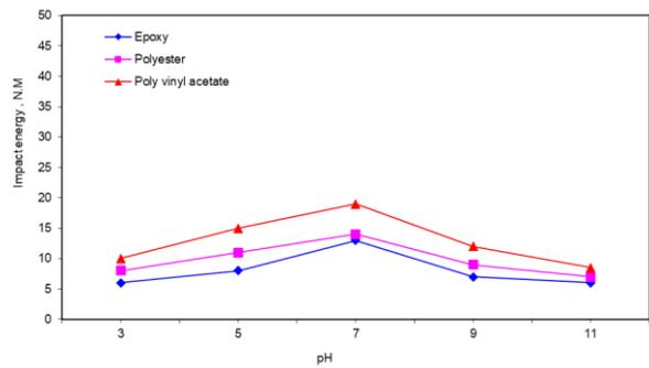
**Figure 15: Effect of pH Values on Impact Energy of the PVC/PVC Sandwich Plates with 0.95 Wt.% Glass Fiber and 2.5 mm from Different Adhesives Thicknesses at 4 hrs.**
