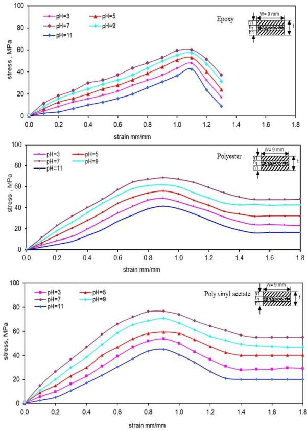
**Figure 8: Effect of pH Values at 2 hrs. on the Stress /Strain Diagram of PVC/PVC Sandwich Plates ( $h_2 = 2.5$  mm, 0.95 Wt. % Glass Fiber)**
