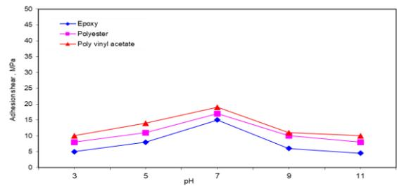
**Figure 18: Effect of pH Values on Adhesion Shear of PVC/PVC Sandwich Plates with 0.95 Wt.% Glass Fiber and 2.5 mm at Different Adhesives Thickness at 4 hrs.**
