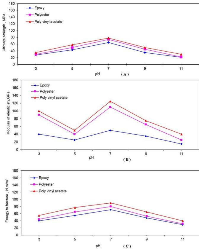
**Figure 13: Ultimate Strength, Modulus of Elasticity and Energy to Fracture Mechanical Tests for the PVC/PVC Plates Blended With 0.95 Wt.% glass fiber as a function of pH Values at 6 hrs.**
