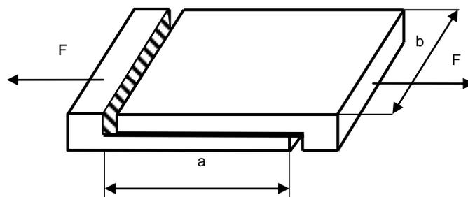
**Figure 4 : Specimens used for the Adhesion Shear Test Method**
