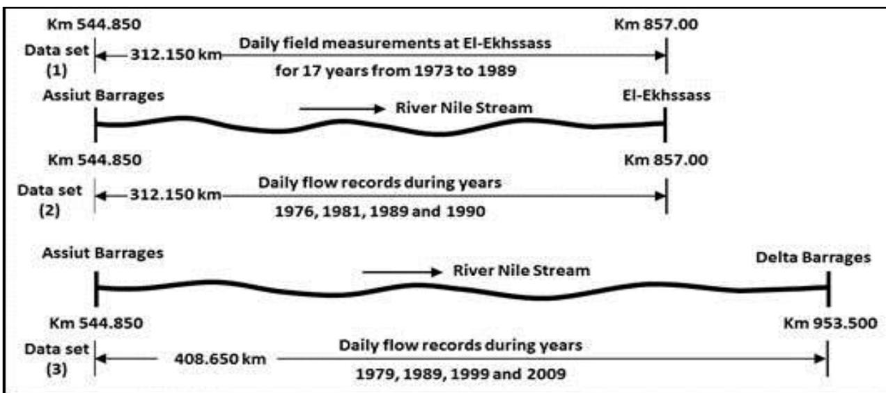
Fig. 5: Downstream boundaries for the three hydrological data sets.
