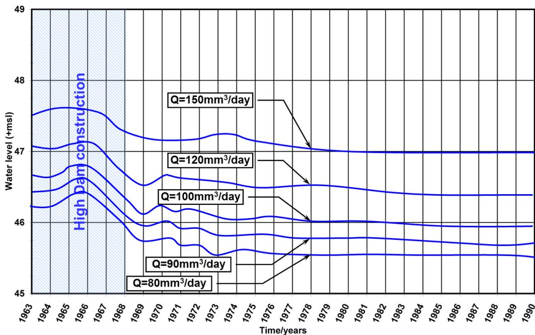
Fig. 1: Water Stage Decline D.S Assuit Barrages directly after HAD Construction (Source: NRI Data Base, 2022 [3]).
