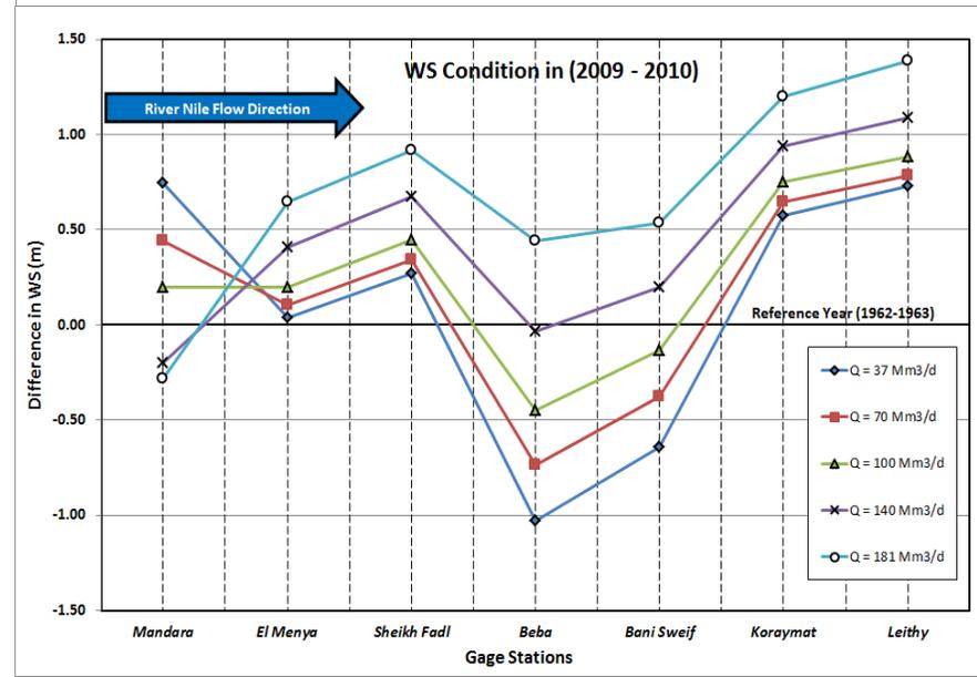
Fig. 8. Development of Water surface profile fluctuations between Years 1979 and 2010 for the five discharge cases compared with 1962-1963.
