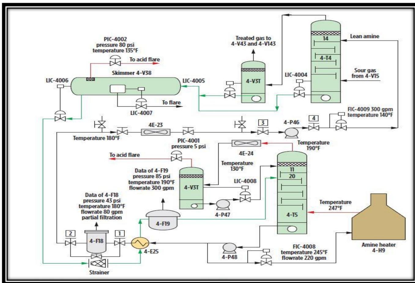
Fig.2. 1 The actual amine unit process flow diagram [8].
